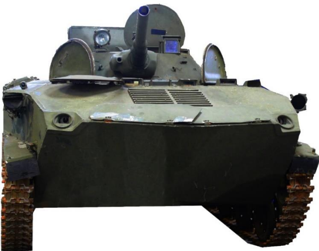
Figure 4: BMP1 at the Defence Academy Shrivenham. Note the two firing ports on the front of the hull.
