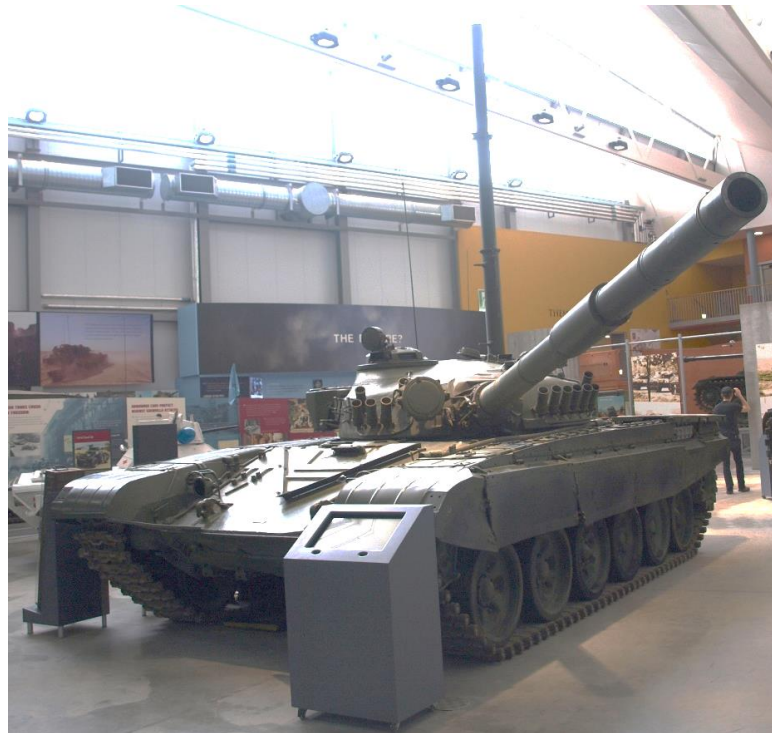
Figure 6: T72 at the Tank Museum, Bovington. Of note is the 5m high snorkel used to allow the vehicle to deep wade.
