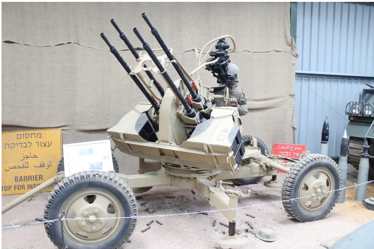
Figure 1: ZPU4 in desert camouflage colour - ex-Iraqi now housed at the military museum at Armouredgeddon in Leicestershire. Having quad 14.5mm machine guns, this was long obsolete for use against attack aircraft but had some utility against helicopters and was also highly useful against ground targets as US Rangers found out during the drop to seize the Port Sallines airport in Grenada in 1983
