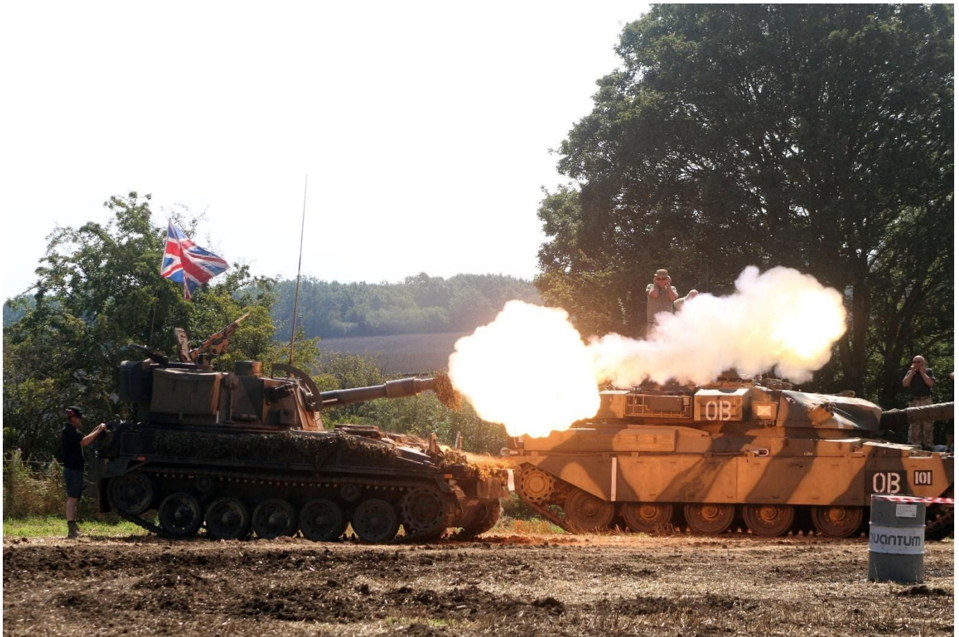
Figure : An Abbot 105mm gun firing at Tanks, Trucks and Firepower 2019. In the background is a Chieftain. The FV433 Abbot is a member of the FV432 series and was replaced by higher firepower 155mm armed vehicles such as the M109.
