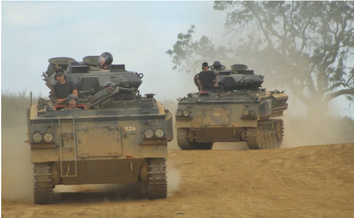
Figure 2: FV432/30s converted to paintballing vehicles (although other than the different muzzle none of the changes are visible from this angle) at Armouredgon. These are Mark 2 versions, identifiable by the exhausts running down the side of the vehicle instead of over the roof (where it could burn passengers).
